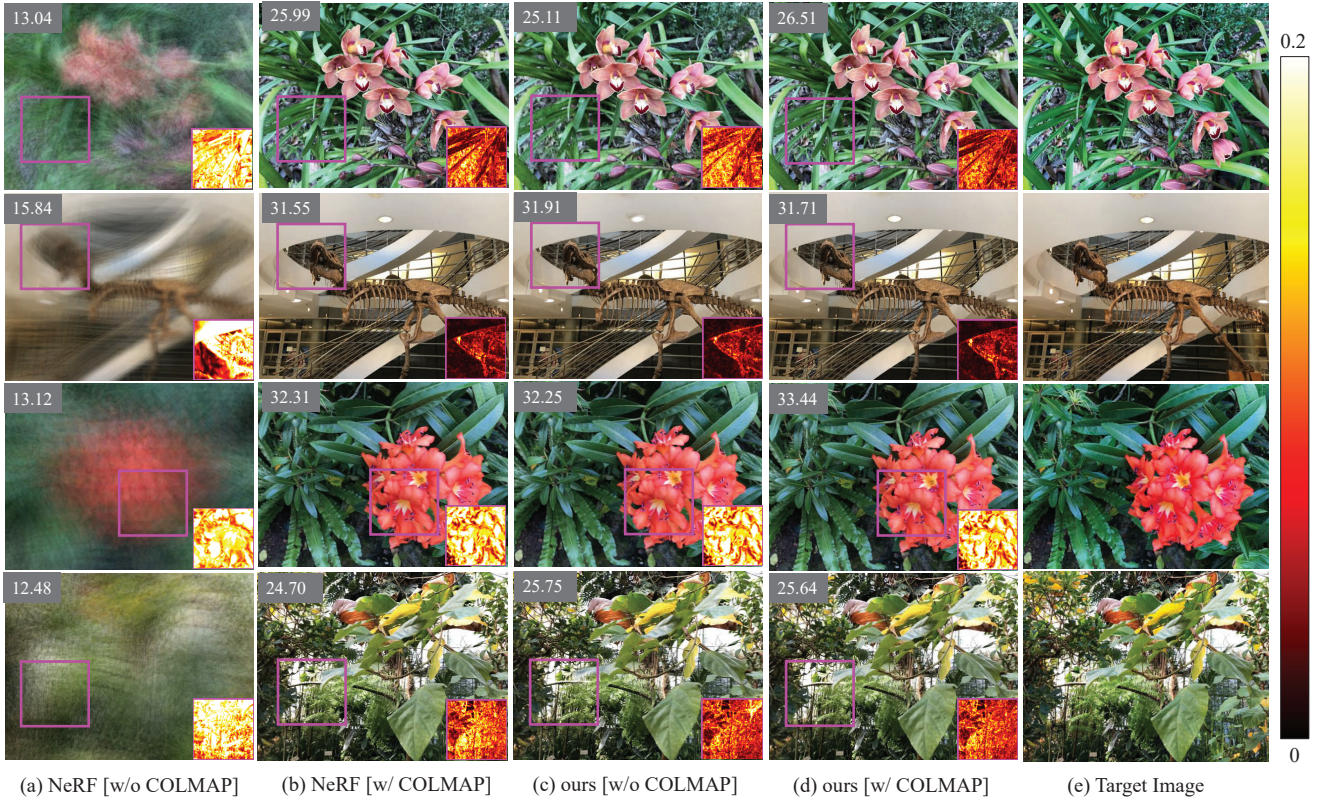
Figure 7. Comparison of NeRF [13] and our approach using LLFF [12] dataset. The first two columns of images show results of NeRF without or with intrinsic and extrinsic camera parameters. We use COLMAP [17] for the camera initialization. The third and fourth columns show rendered images using our approach with the same configuration. Our self-calibration approach shows consistent results regardless of using the camera prior. For each subfigure, PSNR is shown on the upper left.
